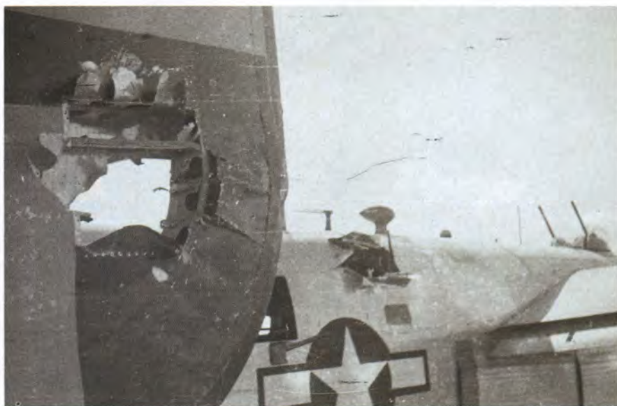
This B-24 made it back to base after the group’s first encounter with rocket-armed fighters. One rocket left this gaping hole; another killed both waist gunners. The surviving crew members were sent home after only one mission. The lack of paint on this “silver-sided” plane types it as a replacement aircraft.
